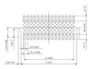
Note: Shaded area must be free of any electrically conductive traces to avoid contact with soldered pin header terminations.
